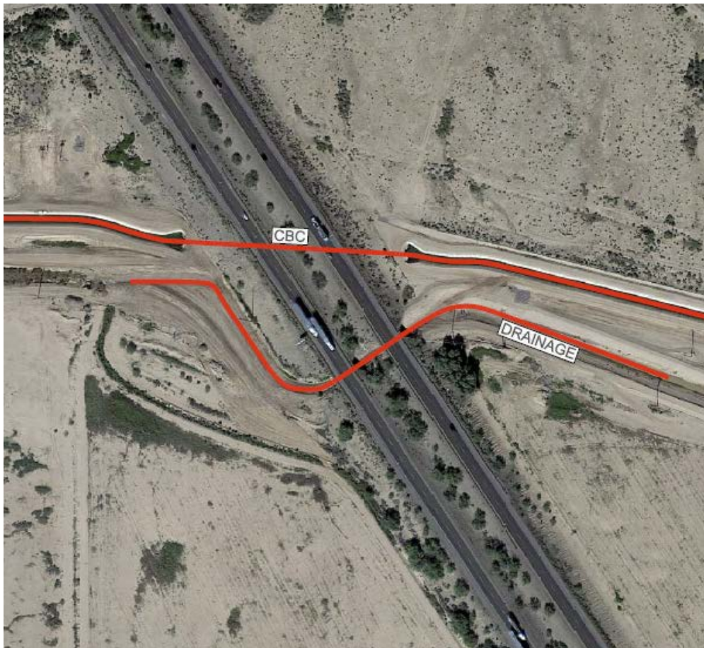
Figure 6: Casa Blanca Canal and Drainage Channel Impacts south of Casa Blanca Road.
